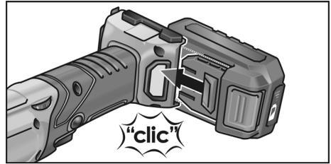
1. Press the charged battery into the power tool until it clicks into place.
