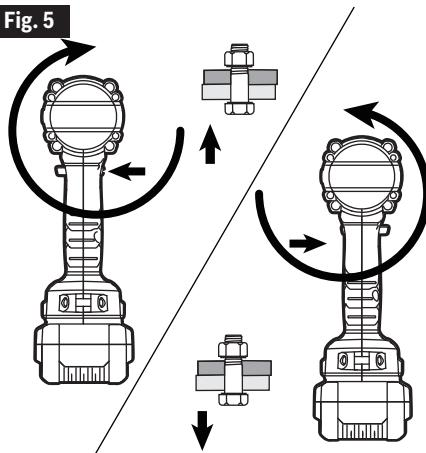
**NOTICE:** The impact wrench will not run unless the direction-of-rotation selector is engaged fully to the left or to the right.
