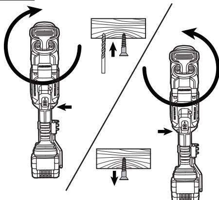
**NOTICE:** To prevent gear damage, always allow the tool to come to a complete stop before changing the direction of rotation.
